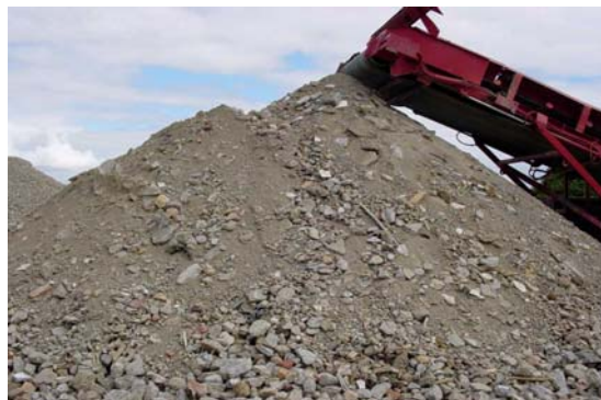
Crushed concrete product, Ward Resource Recovery, Auckland
